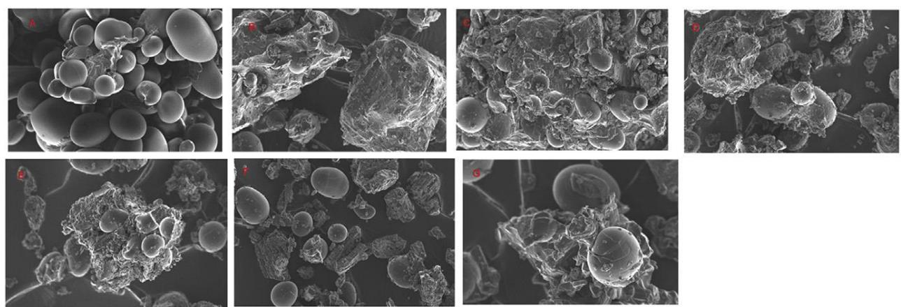
Scanning electron micrographs of (A) native BGN starch, BGN starch-catechin complexes modified through; (B) microwave method using alpha cyclodextrin, (C) microwave method using beta cyclodextrin, (D) kneading method using alpha cyclodextrin, (E) kneading method using beta cyclodextrin, (F) co-evaporation method using alpha cyclodextrin, (G) co-evaporation method using beta cyclodextrin.
